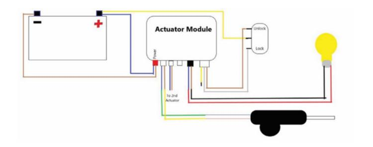
NOTE: MULTIPLE ACTUATORS CAN BE WIRED INTO EACH OUTPUT EACH ACTUATOR OUTPUT HAS MAX OUTPUT OF 20 AMPS IN THE DITCH ACTUATORS HAVE MAX DRAW OF 4.5 AMPS
