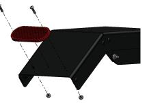
Note: intended to be left and right, install red reflectors to be pointed to the rear, amber to be pointed to the front while in use.
