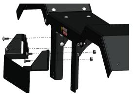
Note: if using dolly fenders with another brand of dollies with a 2" frame, install the 2" adapter bracket PN: ITD25462 (steel 2" adapter bracket), or ITD25488 (ALUMINUM 2" ADAPTER BRACKET)
